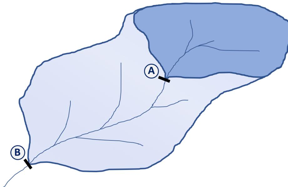
**Figure 4. Example watershed showing two pond dams (black lines labeled “A” and “B”) and their treated areas (shades of blue). Stream flow is from upper right to lower left.**
